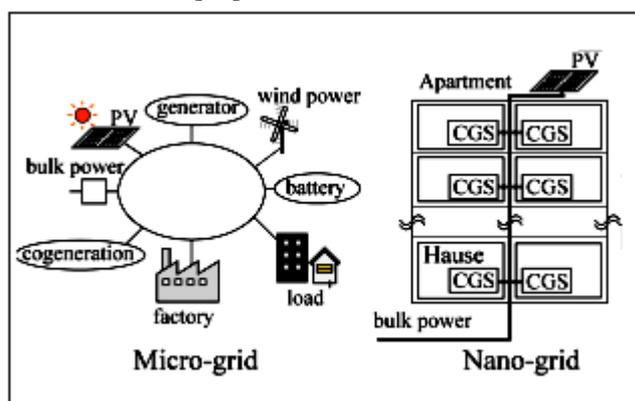
**Fig 1 :** Microgrid and Nanogrid System
